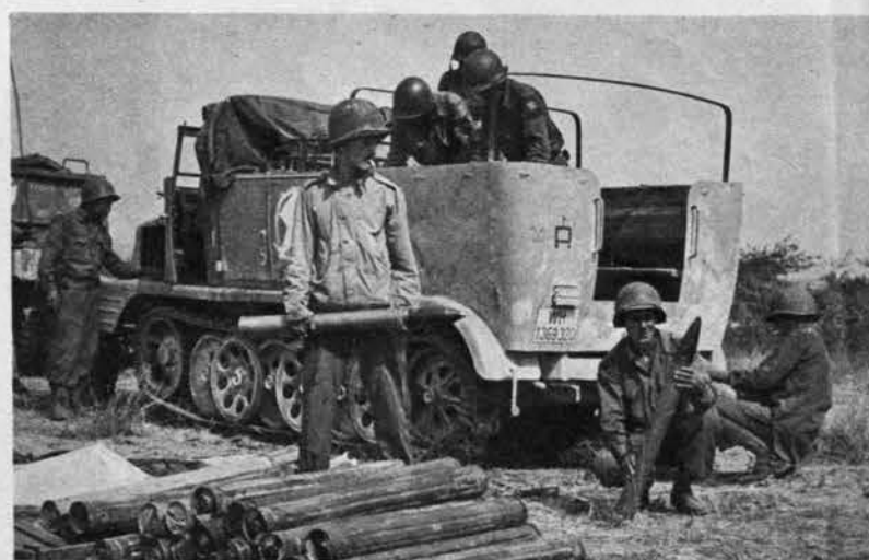
Yanks in Italy captured this German half-track loaded with 88-mm. shells. Like U.S. half-tracks, it has pair of unpowered truck wheels in front. Its overlapping bogie wheels are unique German feature.
